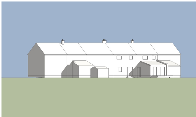
3D Shadow Model - Rear Terrace (South) Elevation View Image taken at Time 08:00am & Date 21 Mar
