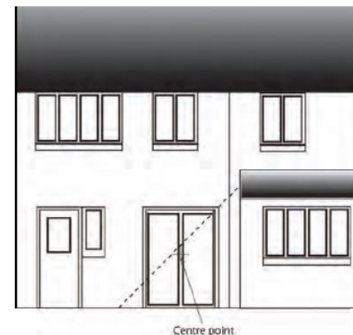
Diagram 2 - 45° Assessment in both elevation and plan form. As the centre point would be within the 45° splay then the proposal would fail the test
