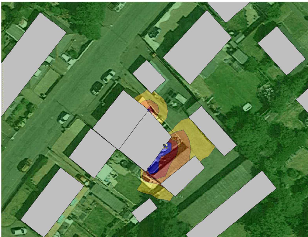
Figure 6.1 Plan view of noise propagation in 3D noise mapping model
