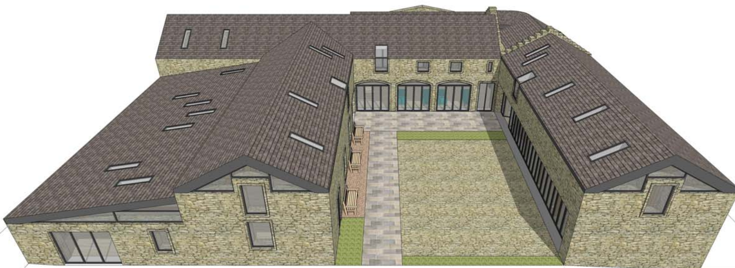
New flooring throughout, windows and doors to existing openings, new roof sympathetic to the original form and landscaping to aid flexible use of courtyard
